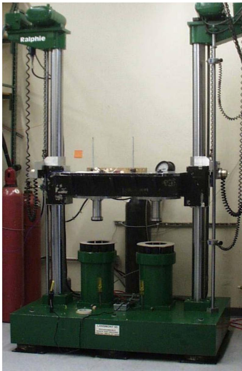
**Figure 14: Programmable Shock Test Machine**
